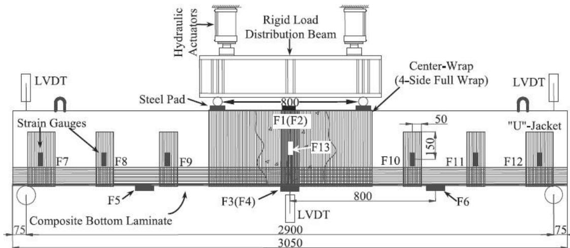
Figure 8. Retrofit schemes for CFRP retrofitting [5]
