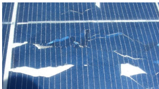
Figure 5. Shattered c-Si cell
