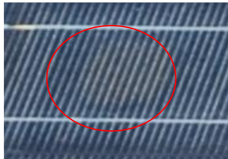
Figure 23. Module C cell center browning
