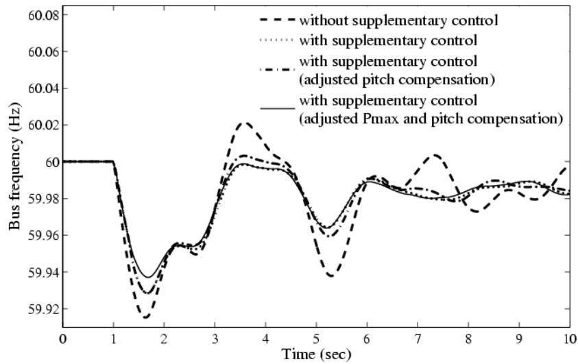
Figure 6.23 Frequency at bus 32729 (69 kV) for Case B
