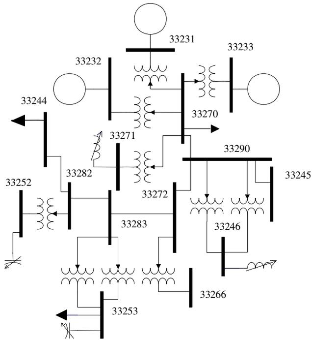
Figure 6.4 Single line diagram showing the bus structure near a generator with highest participation factor
