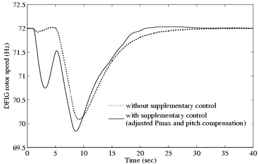
Figure 6.27 Effect of wind ramp down on DFIG rotor speed for the cases with and without supplementary control
