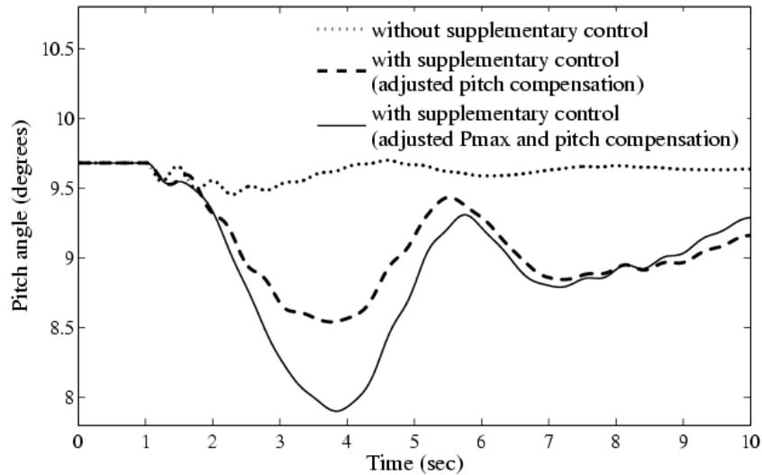
Figure 6.17 Pitch angle of DFIG at bus 32672 with and without supplementary control
