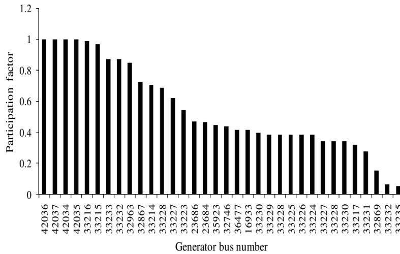
Figure 6.2 Participation factor corresponding to the generator speed state for the dominant mode with beneficial effect on damping
