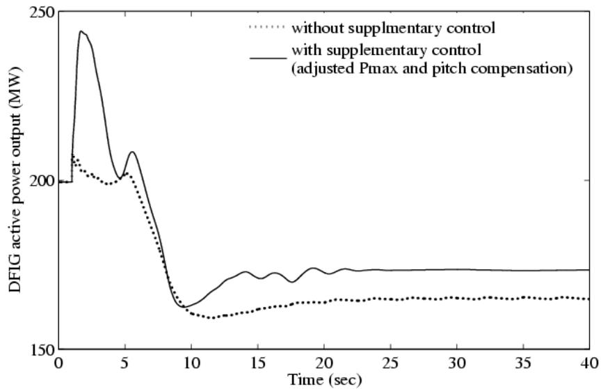
Figure 6.29 Effect of wind ramp down on DFIG active power output for the cases with and without supplementary control
