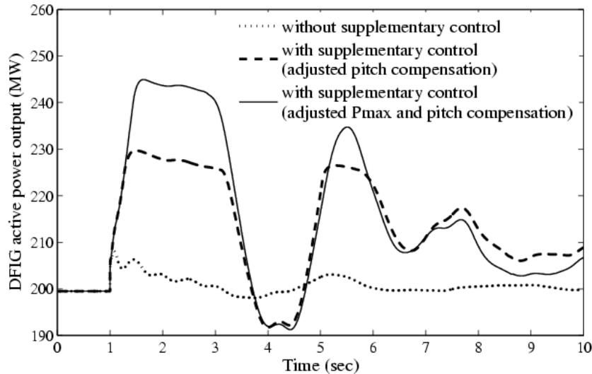
Figure 6.15 Power output of DFIG at bus 32672 with and without supplementary control
