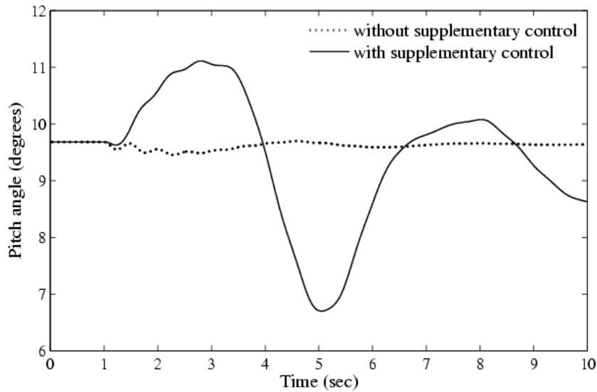
Figure 6.13 Pitch angle of DFIG at bus 32672 with and without supplementary control
