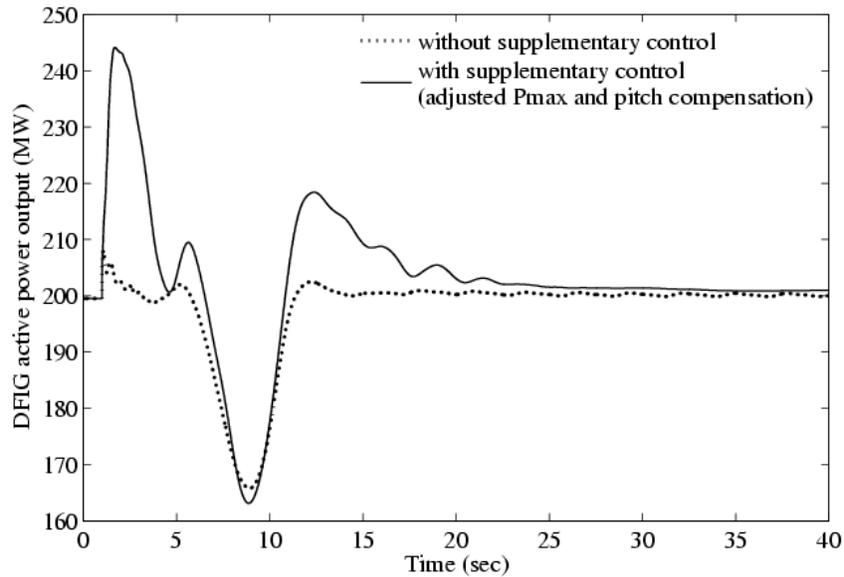
Figure 6.28 Effect of wind gust down on DFIG active power output for the cases with and without supplementary control
