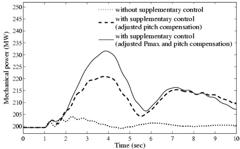
Figure 6.18 Mechanical power of DFIG at bus 32672 with and without supplementary control
