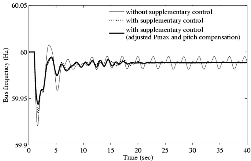
Figure 6.25 Frequency at bus 24222 (161 kV) for Case B
