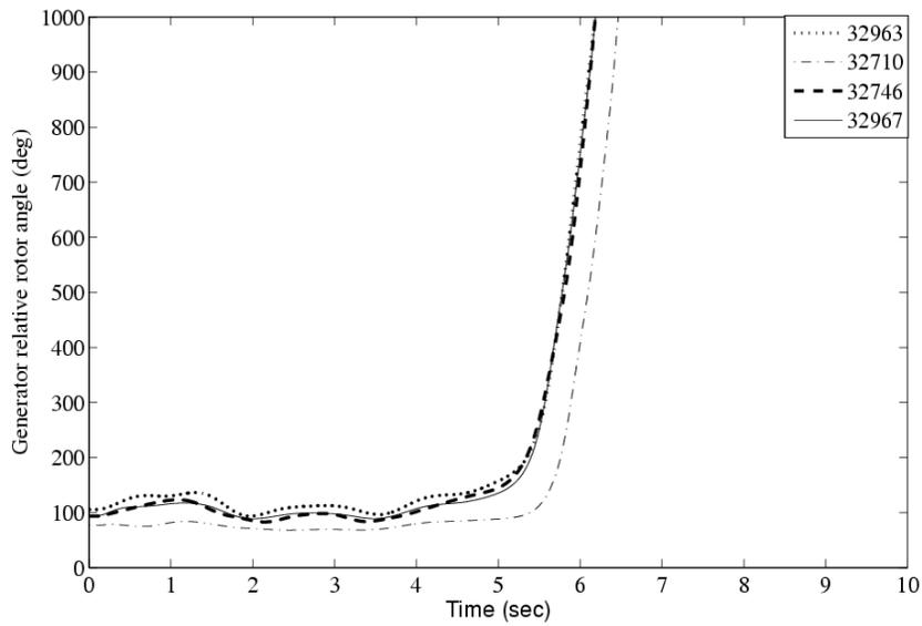
Figure 6.8 Generator relative rotor angle for machines accelerating in Case C
