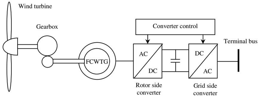
Figure 2.3 Full converter wind turbine generator
