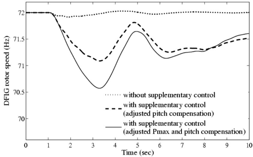
Figure 6.16 Rotor speed of DFIG at bus 32672 with and without supplementary control
