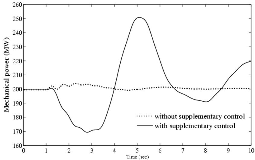
Figure 6.14 Mechanical power of DFIG at bus 32672 with and without supplementary control
