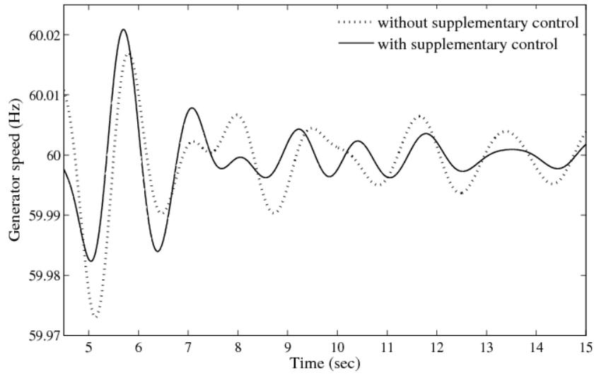
Figure 6.30 Generator speed for the bus 33232 for the Case B
