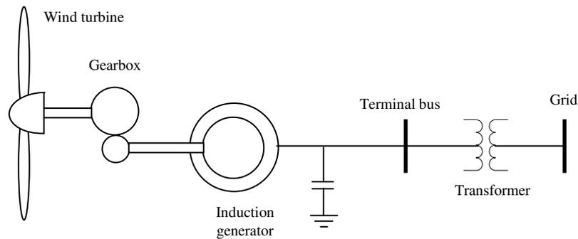
Figure 2.1 Fixed speed wind turbine generator
