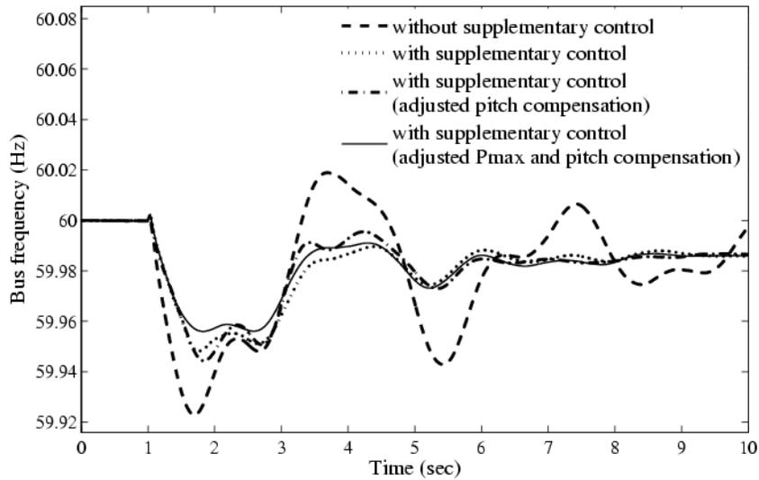
Figure 6.24 Frequency at bus 32729 (69 kV) for Case C
