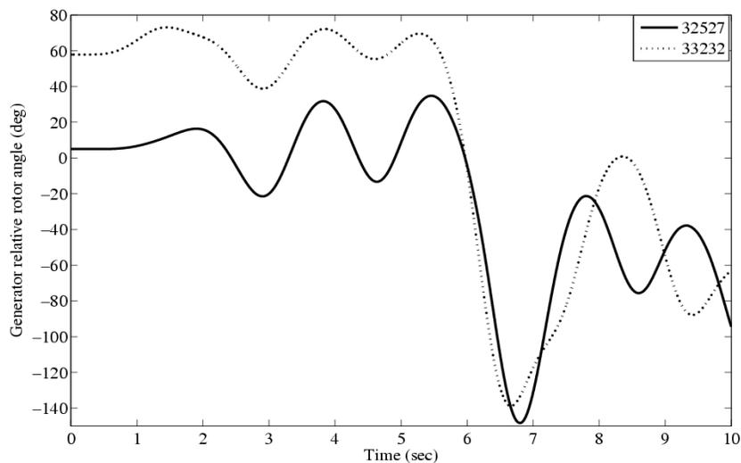
Figure 6.9 Generator relative rotor angle for machines decelerating in Case C
