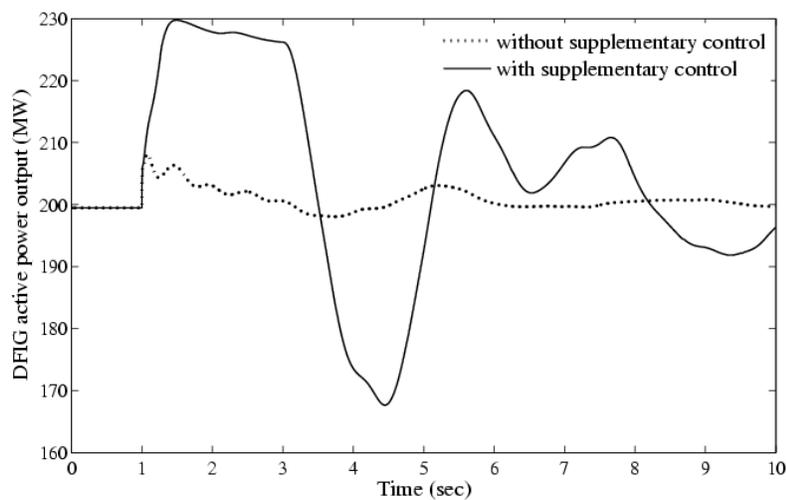
Figure 6.11 DFIG power output at bus 32672 with and without supplementary control
