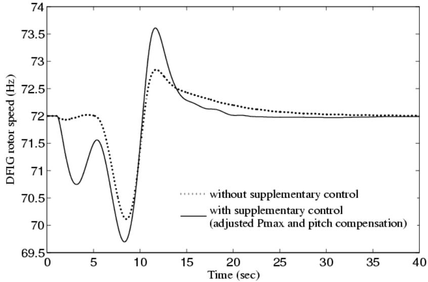
Figure 6.26 Effect of wind gust down on DFIG rotor speed for the cases with and without supplementary control
