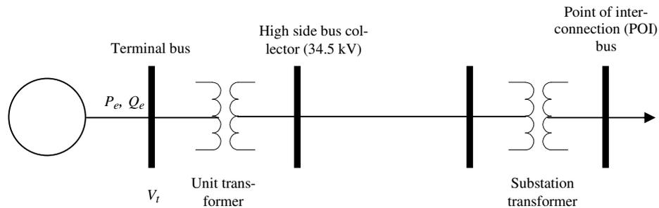
Figure 3.1 Power flow model of wind farm [46]
