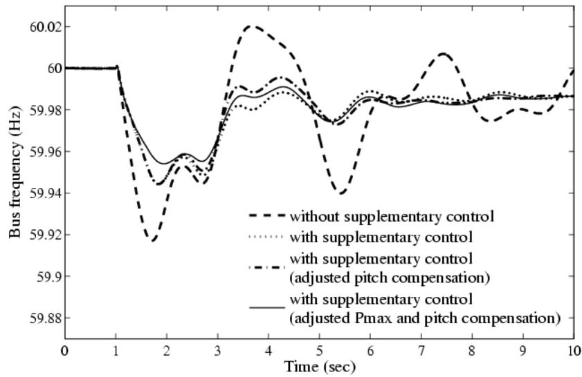
Figure 6.22 Frequency at bus 24222 (161 kV) for Case C
