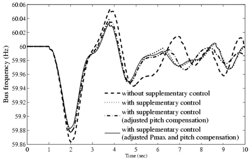
Figure 6.19 Frequency at bus 32969 (345 kV) for Case B
