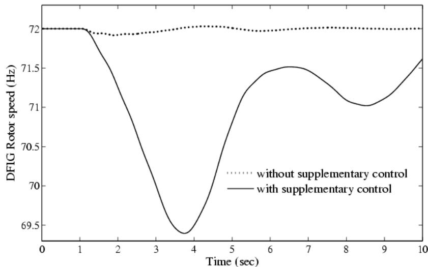
Figure 6.12 Rotor speed of DFIG at bus 32672 with and without supplementary control
