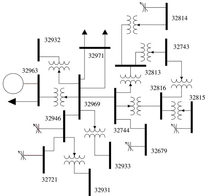
Figure 6.6 Single line diagram showing the bus structure near the generator 32963 with high participation factor
